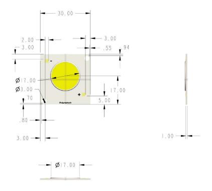
Dimensions are in mm. Tolerances unless otherwise specified: +.13  $x^{\circ} +1^{\circ}$
